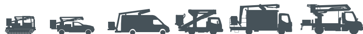
TRACK MOUNTED PICK-UP MOUNTED VAN MOUNTED CHASSIS MOUNT TRUCK MOUNTED INSULATED PLATFORM
